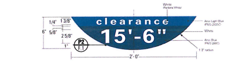
3 Detail - Canopy Clearance Sign scale: 1" = 1'-0"
